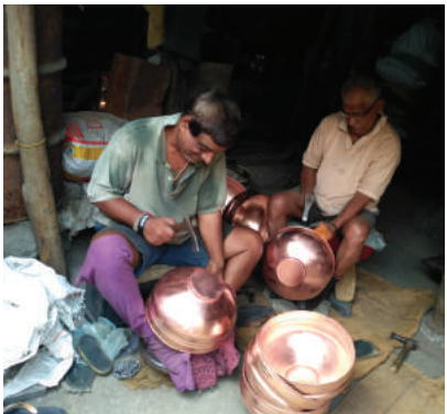
Copper plates are placed against an iron bolt and hammered to give them a 'U' shape.
